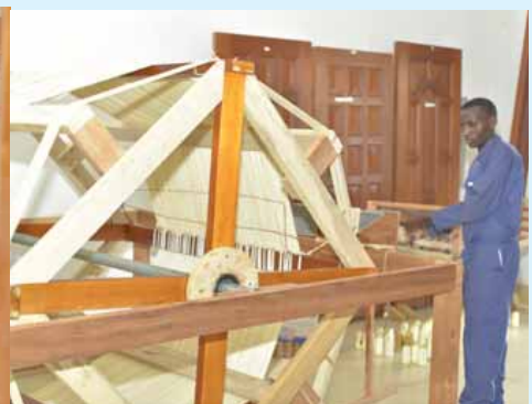
Weaving looms fabricated at the UIRI carpetry workshop
